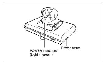
The Communication Terminal turns on after a while. Three indicators on the front of the Communication Terminal and the POWER indicator on the camera light, then only the POWER indicators on both units remain on in green. The launcher menu will appear on the monitor screen and the picture shot by the local camera will also appear in the launcher menu.
